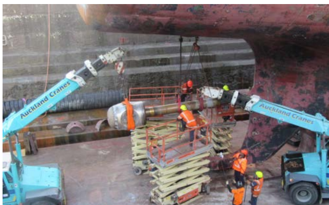
Tomi Maru 87 – Re-fitting propeller shaft following inspection and bearing surface repairs
