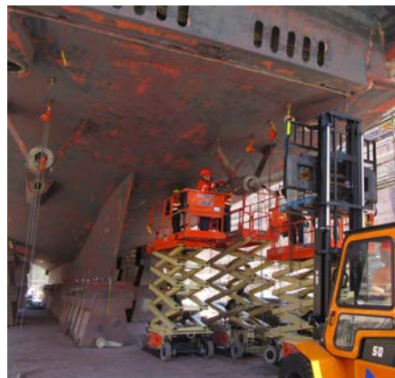
Rudders and propeller shafts removed for survey
